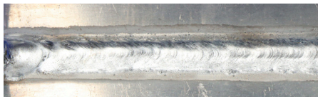
Single Pulse MIG – Using 1.0mm AL5356 Aluminium Wire welding 3.0mm sheet using right to left push technique.
