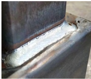
Steel RHS welded with Single Pulse MIG, the person who completed this weld was a Left-hander, so they pushed from Left to right!
