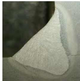
Fillet weld on steel (sectioned and etched with acid) completed using Argon+10% CO2 Shielding Gas
