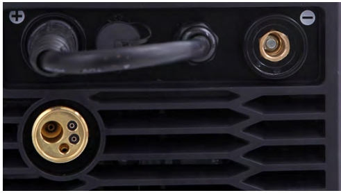
MIG Gun Polarity Cable, Positive (+)
