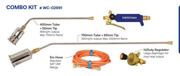
The "all in one" kit with two tube lengths & two tip sizes.
