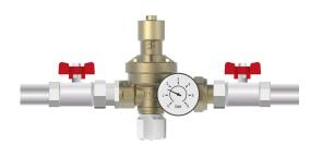
Normally, automatic filling group are installed between two shutoff valves as shown in the figure.
