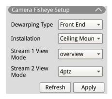
The NVR allows users to adjust dewarping type between Back End dewarping and Front End dewarping depending on the camera's DSP. Select fisheye camera channel and click **Camera Fisheye Setup** on the left to display the settings.
