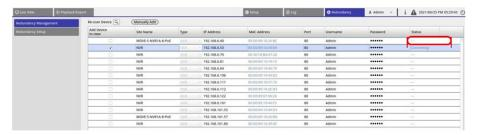
After the setting, there would be three possible situations. One is successfully **monitoring**. The other situation is **backup status activated**. The **offload** situation only happens after the primary NVR failure is fixed.
