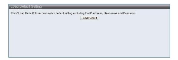
**NOTE!** The Load Factory Default function can only return this PoE switch to the default setting. The User Name, Password and IP Address setting would remain the same.
