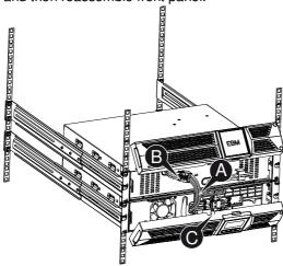
5. After installing the UPS into the rack, the load can then be connected. Please make sure the load equipment is turned off before plugging all loads into the output receptacle.
