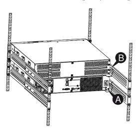
3. Take off the LCD box, and unscrew the internal screws.
