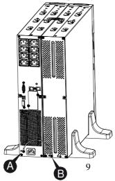
4. Take off the front panel, and connect the battery terminal (A) from UPS to EBM terminal (B) as shown below. Users should remove the small gate (C) on side of the front panel to allow the outlet wire of the EBM to pass through the gate and then reassemble the front panel.
