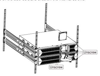
4. Take off the front panel, and connect the battery terminal (A) from UPS to EBM terminal (B) shown as below. Users need to remove the small gate (C) on side of the front panel to allow the outlet wire of the EBM to pass through the gate and then reassemble front panel.
