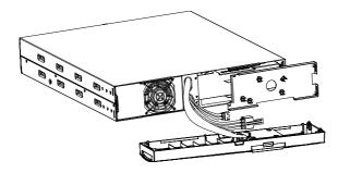
5. Pull the battery pack out onto flat area.
