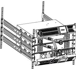
**Note:** Three or more EBMs can be connected to the UPS in the same way as shown above.
