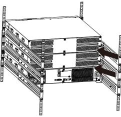
2. Take off the front panel, and connect the battery terminal (A) from UPS to EBM terminal (B) shown as below, then connect the battery terminal (D) from the first EBM to the battery terminal (E) from the second EBM. Remove the small gate (C) on side of the front panel to allow the outlet wire of the EBM to pass through the gate and then reassemble the front panel.
