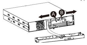
4. Remove the right inner battery bracket.
