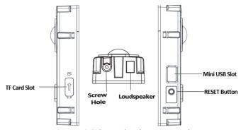
Figure 1-2 Side Panel and Bottom Panel
