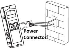
Figure 2-4 Connect Power Cables
