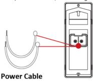
Figure 2-3 Connect Included Power Cables
