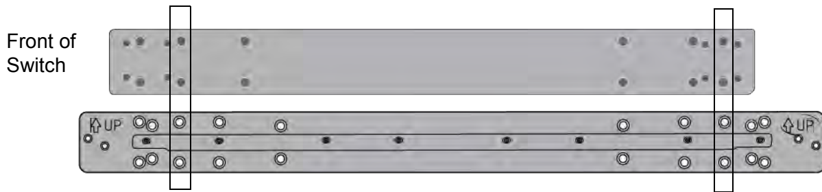
Figure 96. Inner Rail Screw Holes for the x950-28XSQ and x950-28XTQm Switches
