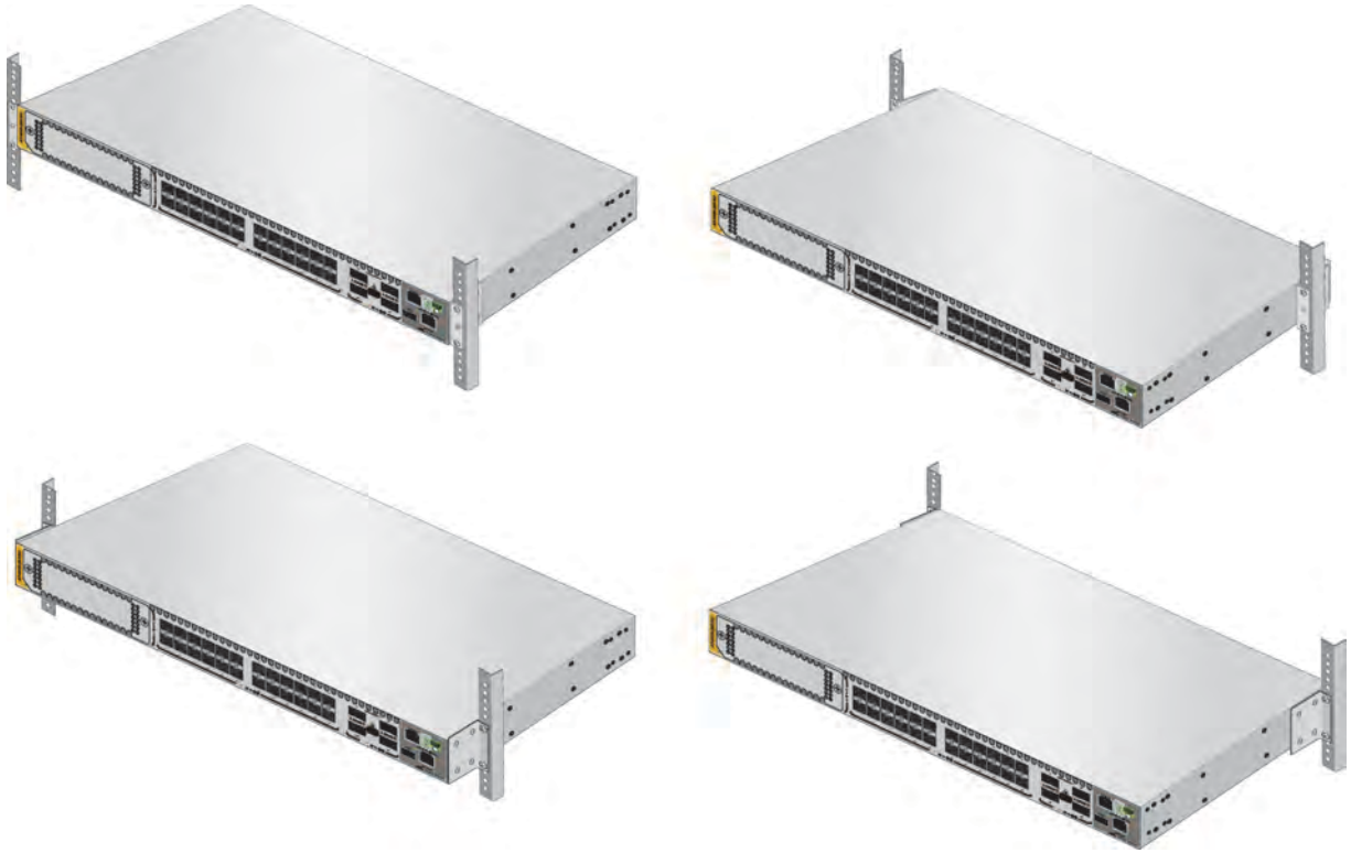
Figure 66. Switch Orientations in an Equipment Rack
