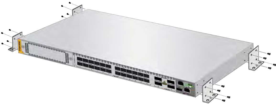
Figure 75. Installing the Brackets to the Switch for Wall Installation
