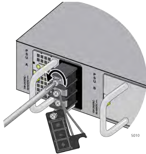
Figure 50. Loosening the Screw for the Negative (+)
