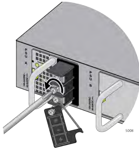
Figure 48. Loosening the Screw for the Negative (-)
