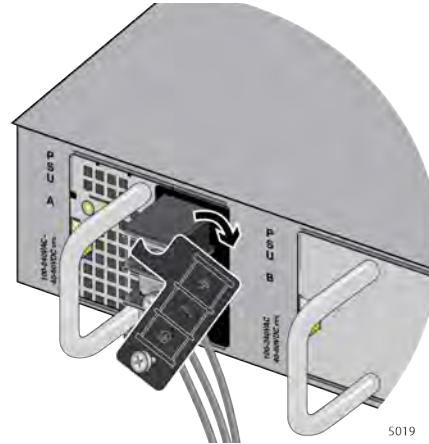
Figure 136. Accessing the Connecting Screws
