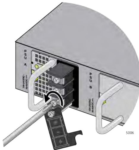
Figure 44. Loosening the Ground Screw
