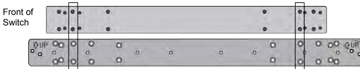
Figure 97. Inner Rail Screw Holes for the x950-52XSQ and x950-52XTQm Switches
