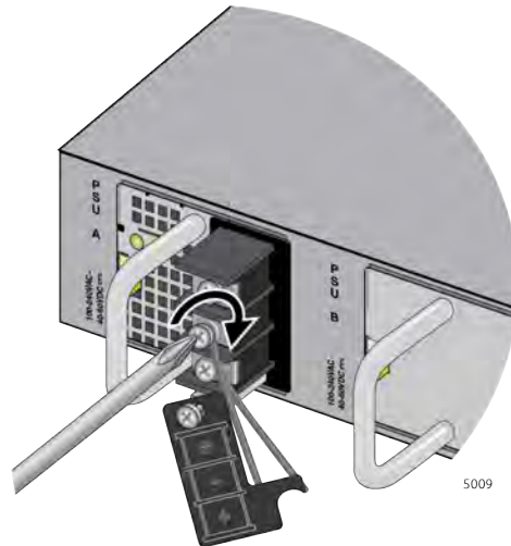
Figure 49. Tightening the Screw for the Negative (-)
