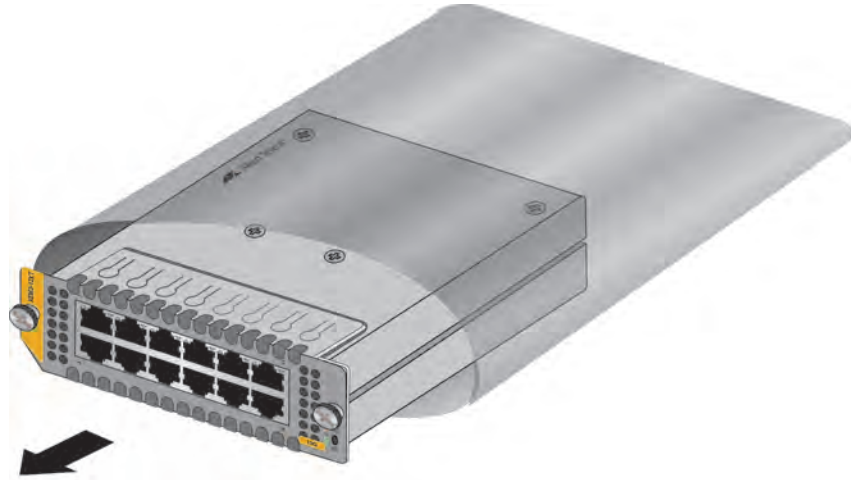
Figure 55. Removing the Ethernet Line Card from the Anti-static Bag
