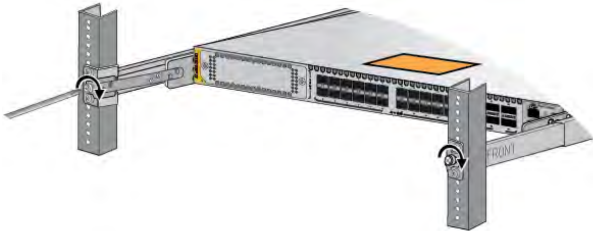
Figure 101. Tightening the Two Screws on the Fixed Brackets
