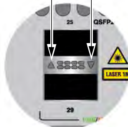
Figure 8. LEDs for Ports 25, 29, 33, and 37 on the x950-28XSQ and x950-28XTQm Switches
