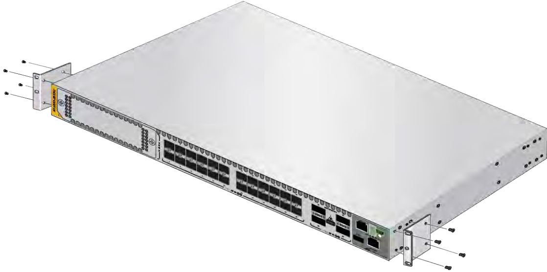
Figure 68. Attaching the Equipment Rack Brackets
