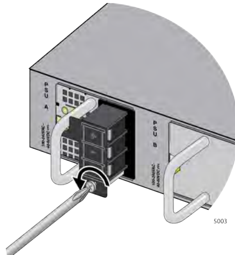
Figure 42. Loosening the Screw for the Panel
