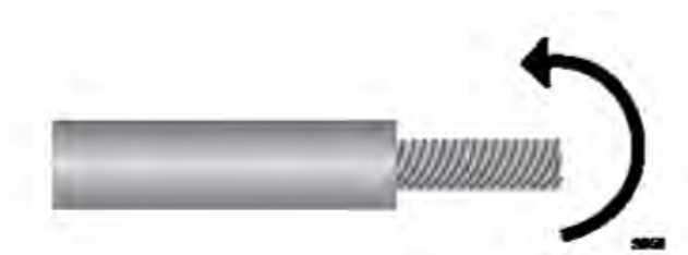
Figure 47. Wrapping the Wire Strands
