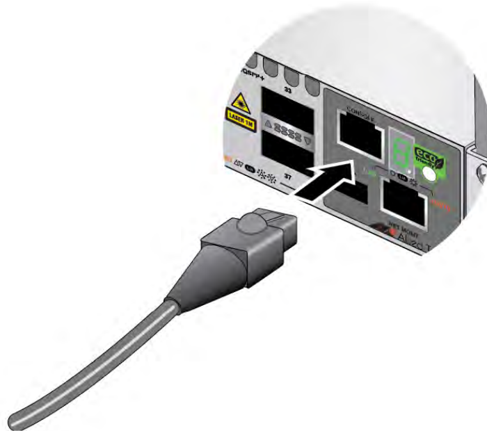
Figure 106. Connecting the Management Cable to the Console RS-232 Port
