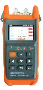
PPM-50 PON Power Meter can perform in-service testing of all PON signals (1310/1490/1550nm) at any spot on the network featuring pass-through design, burst mode and Pass/Warning/Fail assessment function, which can greatly help you evaluate PON signals transmission quality.
