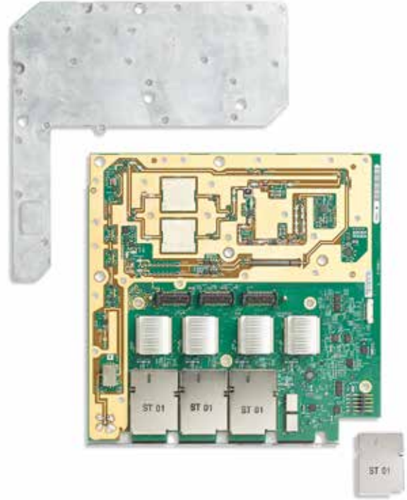
Figure 10. MDO4000C analog board with shields removed clearly shows the RF signal path.
