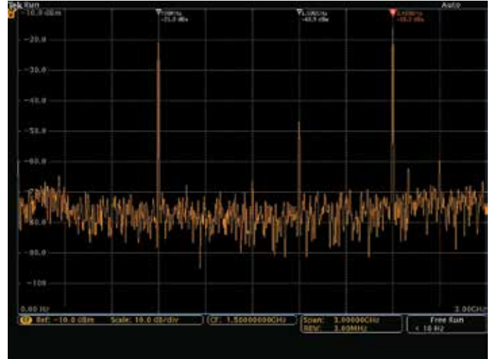
Figure 13. An MDO can capture a signal in both the 900 MHz and 2.4 GHz ISM bands simultaneously.
