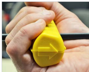
Close the tool onto the cable and pull in the direction of the arrow; clamps tightly — no latch required.
