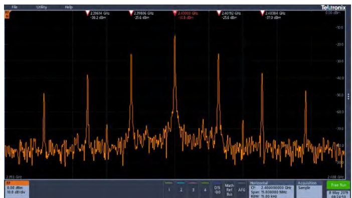
Automated peak markers identify critical information at a glance. As shown here, the five highest amplitude peaks that meet the threshold and excursion criteria are automatically marked along with each peak's frequency and amplitude.
