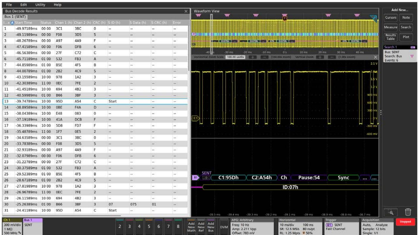
For firmware engineers, the Results Table format may be more useful. This time-stamped display of bus activity can be easily compared to software listings, and allows easy calculation of the execution speed.
