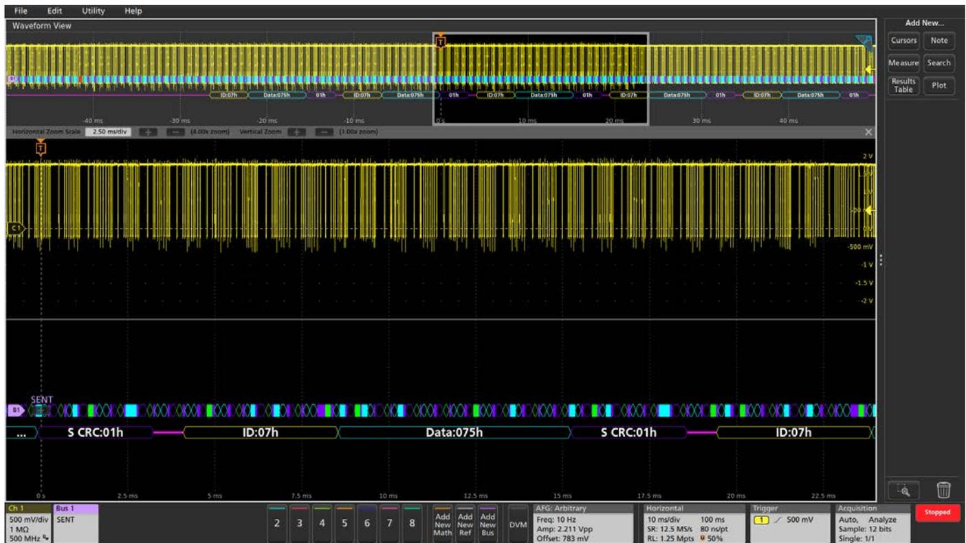
The decoded SENT bus can display both fast and slow channel packets in a single waveform display, with the slow channel packets shown below the fast channel packets.
