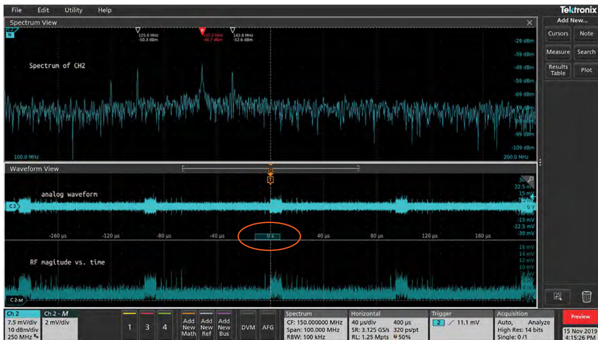
FIGURE 13. The center trace is the time-domain waveform from the H-field probe. The spectrum view (top) gives the frequency content corresponding to the spectrum time indicated by the blue block below the waveform (circled in orange). The RF Amplitude vs. Time trace (bottom) shows a repetitive RF burst.
