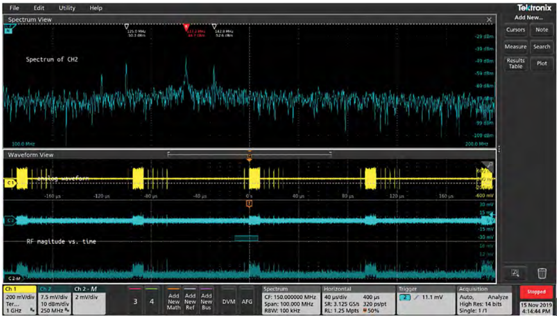
FIGURE 14. Probing signals with a passive probe on Channel 1 (yellow) uncovers a signal that correlates with the RF (cyan).
