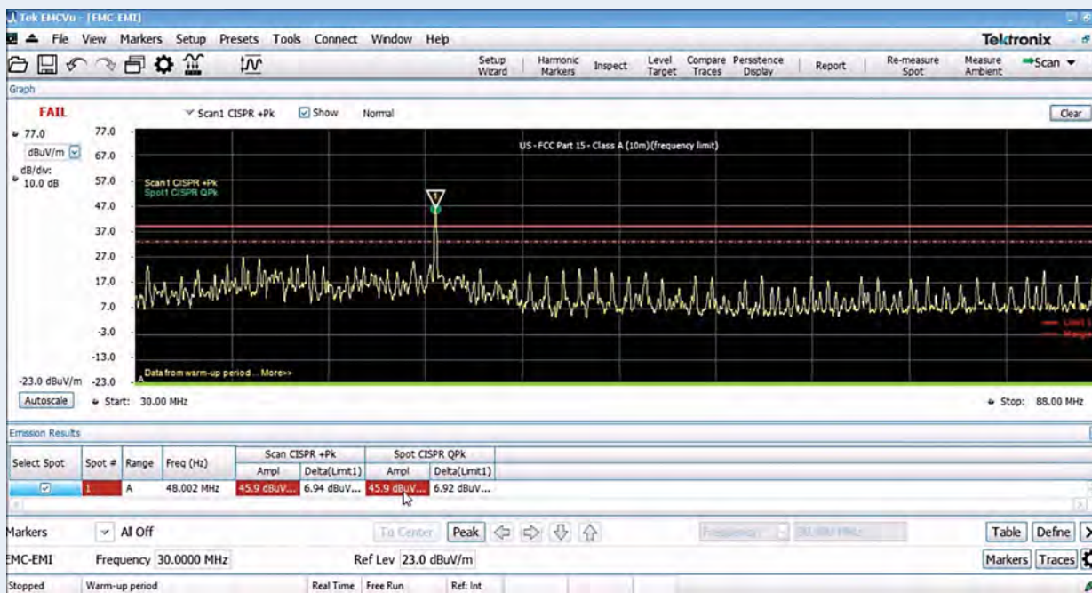
FIGURE 3. Comparison of peak detection and quasi-peak detection in plot and tabular formats on a continuous wave (CW) signal. The plot was generated using EMCvU pre-compliance software and a Tektronix RSA306B Spectrum Analyzer.
