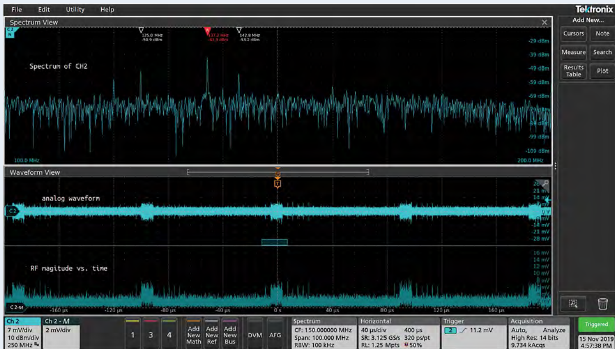
FIGURE 10. Spectrum View lets you view time, frequency and amplitude on the same screen with measurement data uniquely available for each domain.
