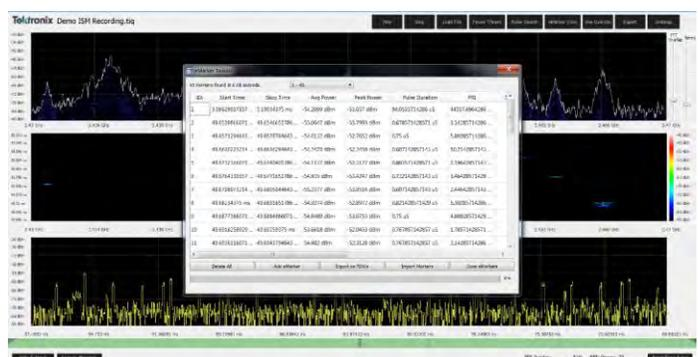
The pulse analysis application license illustrated above enables you to search for pulses and return all results with start/stop time, average power, peak power, pulse duration, PRI and start/stop frequencies. Pulse parameters can be exported to a CSV file for use with other tools.
