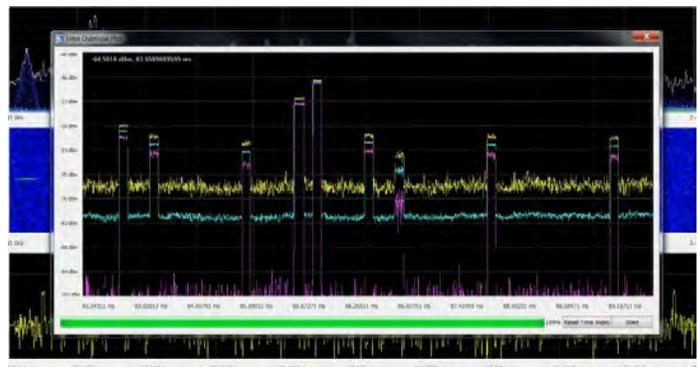
The Time Overview display in application license SMARK provides the +peak (yellow), -peak (purple) and average (blue) traces of the entire recording in a single snapshot. You can use the mouse to identify an area of interest, and this portion of the time record is used to set the start and stop points of the detailed analysis. In this way, you can easily zoom in on active regions, quickly examining areas of interest.
