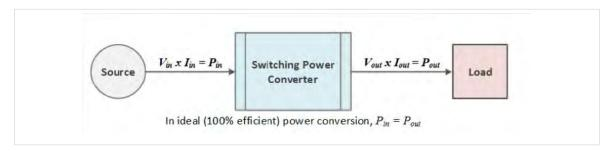
Figure 2: Ideal power conversion efficiency [1].
