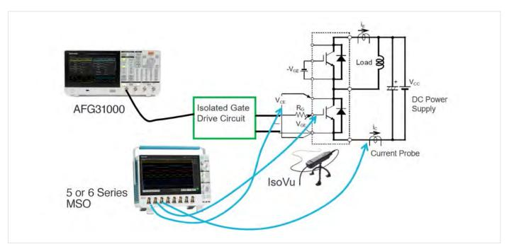
Figure 9: Double Pulse Test Setup.
