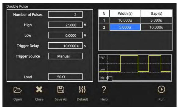
Figure 15: Double Pulse Test settings on the AFG31000.
