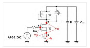
Figure 14: Scope measurements test points.
