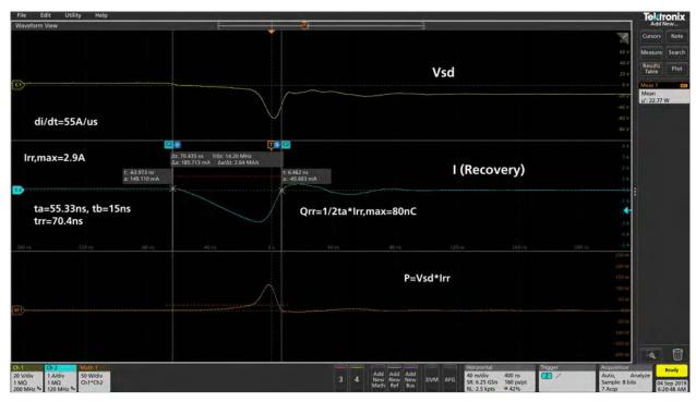
Figure 21: Reverse recovery waveforms.
