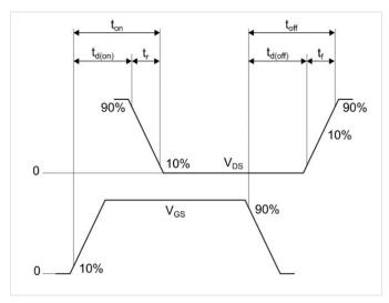
Figure 17: Switching Time Standard Waveform [5].
