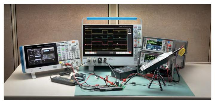
Figure 12: Double Pulse Test setup.
