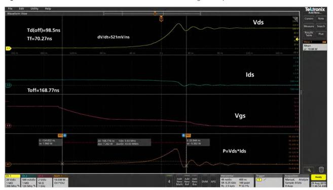
Figure 19: Turn-off parameters waveforms.
