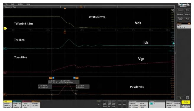
Figure 18: Turn-on parameters waveforms.
