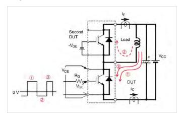
Figure 7: Current Flow using IGBTs as DUTs.
