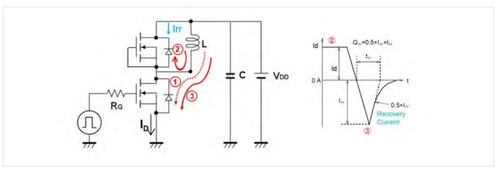
Figure 20: Diode reverse recovery.
