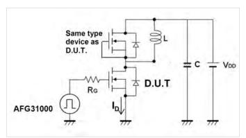
Figure 5: Double Pulse Test circuit.
