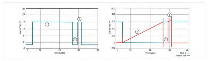
Figure 8: Typical Waveforms of the Double Pulse Test.
