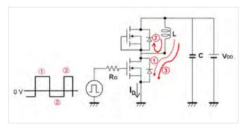
Figure 6: Current Flow with MOSFETs as DUTs.
