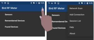
**Network Scan** — This menu option scans the WiFi network the android device is connected to for any Bird devices connected to the same network.
