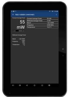
Figure 1 Digital Power Meter Display, 5000-NG
