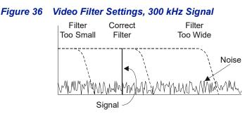
Except for average power and VSWR measurements, all WPS measurements rely on a variable video filter to improve accuracy. This filter can be set to either 4.5 kHz, 400 kHz, or full bandwidth (10000kHz). It should be as narrow as possible while still being larger than the demodulated signal bandwidth (video bandwidth). Narrowing the filter limits the noise contribution caused by interfering signals. Listed below are some common modulation schemes and the appropriate video filter.
