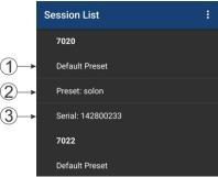
When a power sensor is connected to the Bird RF Meter the first time the Generic Session File (Default Preset if created) is used to initialize the App then a Serial Number Specific Session File is automatically created.
