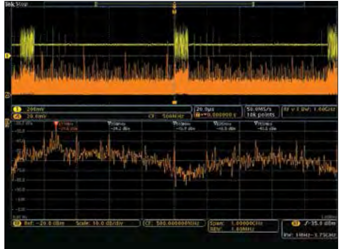
Figure 13. Probing signals with a passive probe on one of the oscilloscope channels uncovers a signal that correlates with the RF.
