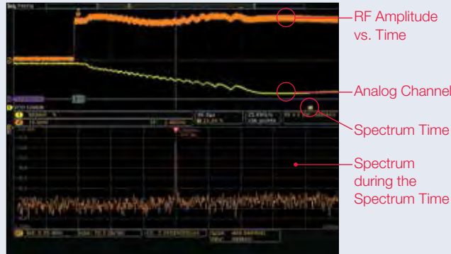
Figure 9. An MDO4000 Series oscilloscope provides a time-correlated view of an oscillator start-up.
