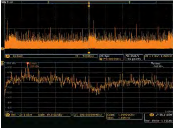
Figure 12. RF Amplitude vs. Time trace shows a significant pulse. The spectrum display shows its frequency content.
