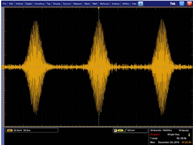
FIGURE 10. Time-domain measurement of a 20ns-wide Gaussian pulse with carrier frequency of 5GHz in the 2nd Nyquist band. A 350MHz-wide digital band-pass filter with 256 taps was used in the oscilloscope to filter out the fundamental and other spurious products.
