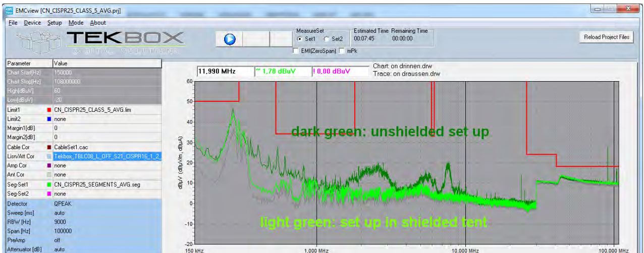
Picture 6: CISPR 25 conducted noise measurement; DUT powered
