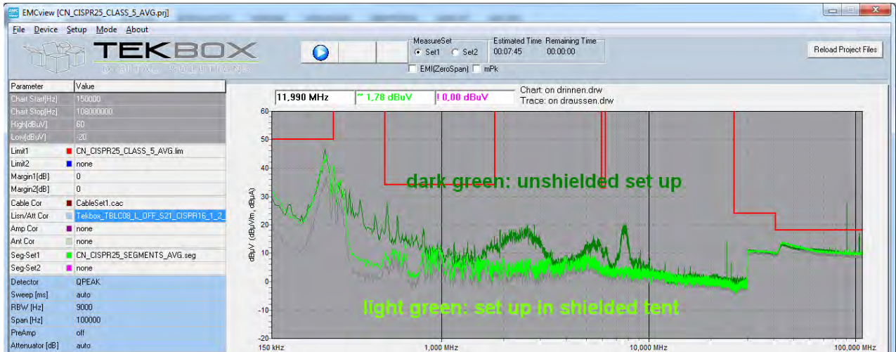
Picture 6: CISPR 25 conducted noise measurement; DUT powered
