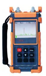
OFI-50A uses optical fiber sensing principle to confirm the target fiber; It can quickly identify deep buried, overhead and pipe fiber cable without any destroy, and provide a simple method for maintenance personnel. Users only need gently knock on cable, when knocking to the target cable, OFI-50 can clearly hear the knock from earphone, which can accurately identify the target cable.
