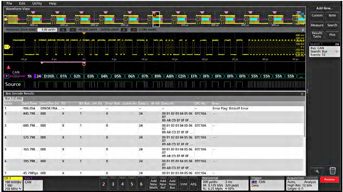
Triggering on a CAN serial bus. A bus waveform provides time-correlated decoded packet content including Start, Arbitration, Control, Data, CRC and ACK while the bus decode table presents all packet content from the entire acquisition.
