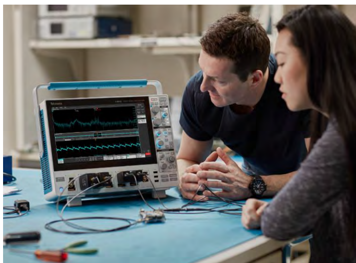
Voltage measurements on a switch-mode power supply showing the ripple voltage on one of the power rails.
