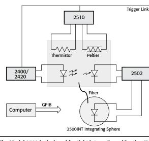
The Model 2502 is designed for tight integration with other Keithley instruments that are often used in LIV test systems for laser diode modules. These other instruments include the Model 2400 SourceMeter<sup>®</sup> and Model 2510 TEC SourceMeter SMU instruments.
