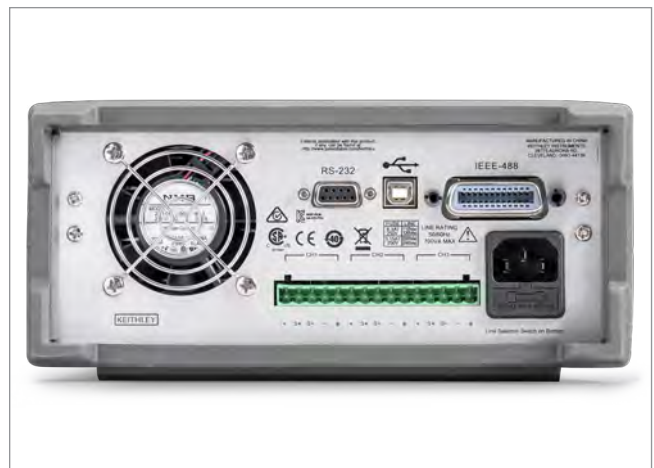
Series 2230G power supplies rear panel showing the USB, GPIB, and RS-232 interfaces and the rear output, source, and sense lead terminal block for all three channels.
