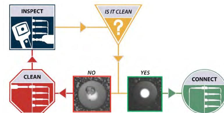
Note: Since contamination is such a big problem with MPO connectors, the best practice is to ensure that all fiber end faces are clean before ever making a connection. This practice, known as "[Inspect Before You Connect](#)" (IBYC) will occur during both the referencing and testing stages, but for purposes of comparison, the time comparisons below will only focus on the testing portion.
