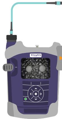
MPOLx with Patch Cord Microscope (PCM)
