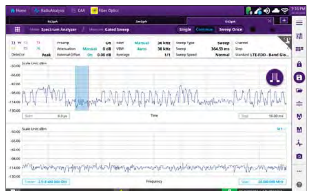
Gated Sweep Spectrum – Spectrum Analysis
