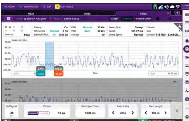
Gated Sweep Spectrum – Gate Time Setting
