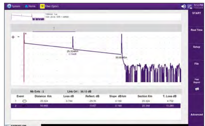
Fiber Characterization – OTDR
