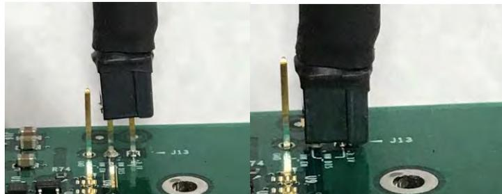
Figure 16: Square Pin Style Sensor Tip Cables
