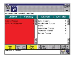
One important error result that is displayed in the summary view is the lost frames result. The FST-2802, using one of its packet generation options, can generate an JDSU test packet. This packet has a sequence number (similar to the TCP sequence number) and a timestamp. This allows the FST-2802 to perform real time QoS and SLA analysis including lost packet rate and round trip delay.
