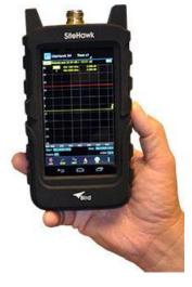
Small and easy to use, this cable/antenna analyser stores thousands of traces for analysis and reporting and offers Measure Match and Distance to Fault functions.
