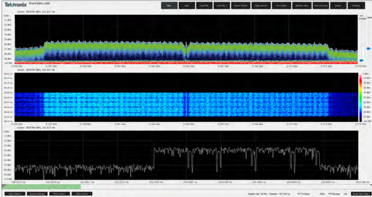
FIGURE 3. Video burst from 5.8 GHz frequency band using I/Q processing.
