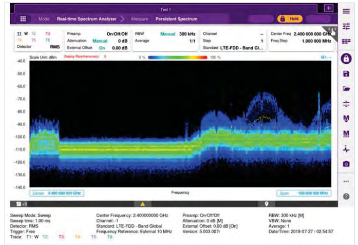
Fig 37: Persistent display showing interference signals in 2.4GHz band.
