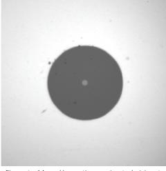
Figure 4a. Manual Inspection requires technicians to judge whether the connector complies with the IEC Standard.
