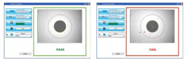
Figure 2. Example of the Proven Inspection and Analysis Software Program FiberChek2 from Viavi
