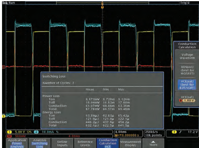
Figure 13. Switching Loss Measurements on an IGBT.
