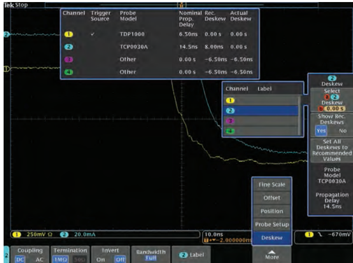
Figure 5. Default Timing Skew between Voltage and Current Probes.
