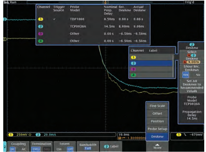
Figure 8. Manual Removal of Timing Skew between Voltage and Current Probes.
