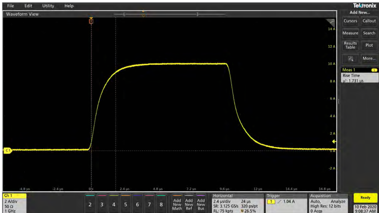
Pulse output performance of the 2610B-PULSE SMU.
