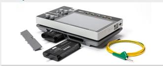
Optional battery pack supports two batteries with an estimated eight hours run time. Batteries can be hotswapped to extend operating time.
