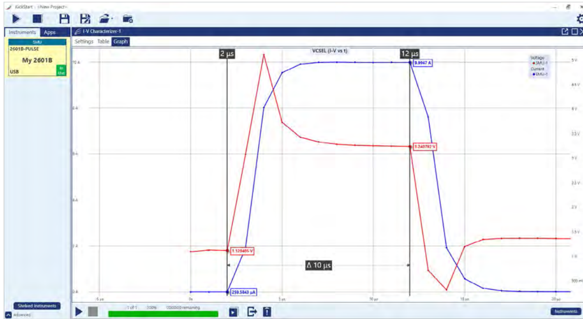
Figure 12. 3 A, 10 \mu s complete waveform measurement
