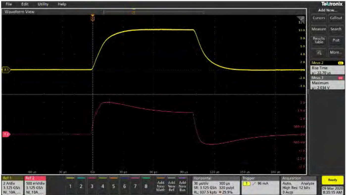
Figure 4. 22 \mu s rise time 10 A pulse on 1 \mu H inductor
