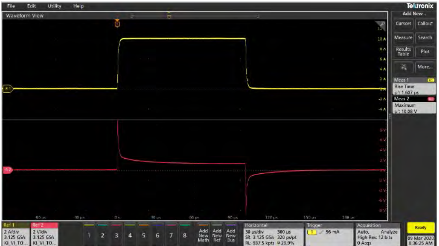
Figure 5. 1.6 \mu s rise time 10 A pulse on 1 \mu H inductor
