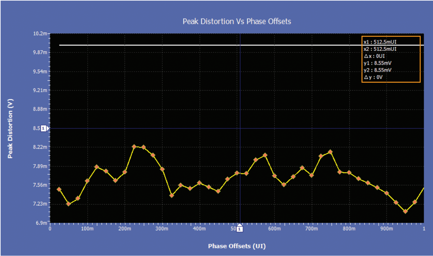
Figure 9. Transmitter Distortion without TX_CLK.
