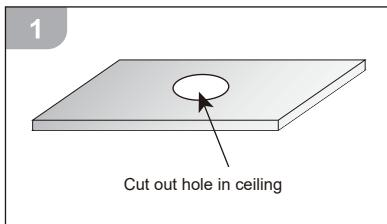
1. Cut out 90mm hole in the ceiling. Ensure there is sufficient clearance in the area where you will position the fitting.
