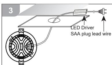
3. Connect fitting to the mains via power plug.
