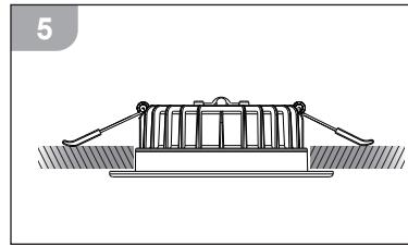
5. Once in place the clips should spring down against the top of the ceiling and support the fitting.
