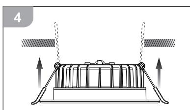
4. Fit the fixture in the ceiling by lifting the springs clips upwards
