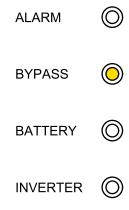
5. Wait approximately 20 seconds until inverter LED turns steady green, the UPS transfers automatically from static bypass mode to normal mode.
