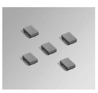
The PFD3215 has a footprint less than  $3.2 \times 2.3$  mm, making this shielded coupled inductor ideal for applications with limited board space. It is designed for use in a variety of circuits including flyback, multi-output buck, SEPIC and Zeta.
