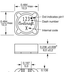
\* For optional tin-lead and tin-silver-copper terminations, dimensions are for the mounted part. Dimensions before mounting can be an additional 0.012 inch (0,3 mm)
