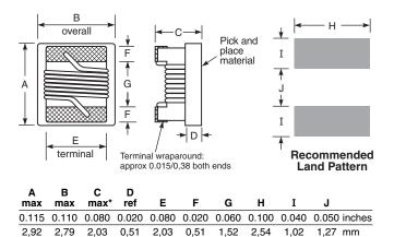
\* Low profile parts: 0.050/1,27 Height dimension (C) is before optional solder application. For maximum height dimension including solder, add 0.006 in / 0,152 mm.
