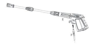
5. Insert the detergent nozzle (J) into the gun (E). Push and turn the detergent nozzle (J) clockwise onto the gun (E) until hand tight to lock it into place. When the pieces are joined properly, you cannot separate the two components by pulling straight out on the gun (E).
