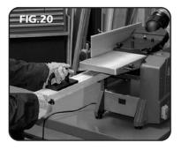
Attach the outlet on the dust extraction port to a suitable dust extractor. This will reduce the amount of airborne dust and health risks associated with the inhalation of particles.
