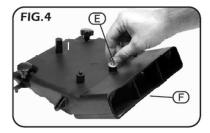
Lower the thicknesser bed using the height adjustment handle (Fig.3) (D) to the lowest point. Insert the dust extraction chute into the feed port and insert the locating lugs on the chute into the holes on the thicknesser bed (G).
