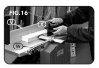
The rear support fence can be tilted 0-45 degrees depending on the chosen application. Unlock lever (Y), select angle, and re-tighten locking lever.
