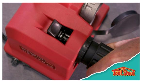
5. Turn the sharpener on and place the sleeve into the sharpening cylinder.
