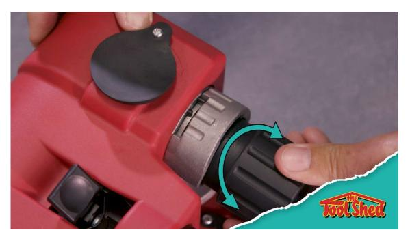
7. Remove the sleeve from the cylinder, rotate it 180°, put it back into the cylinder, and repeat the process.
