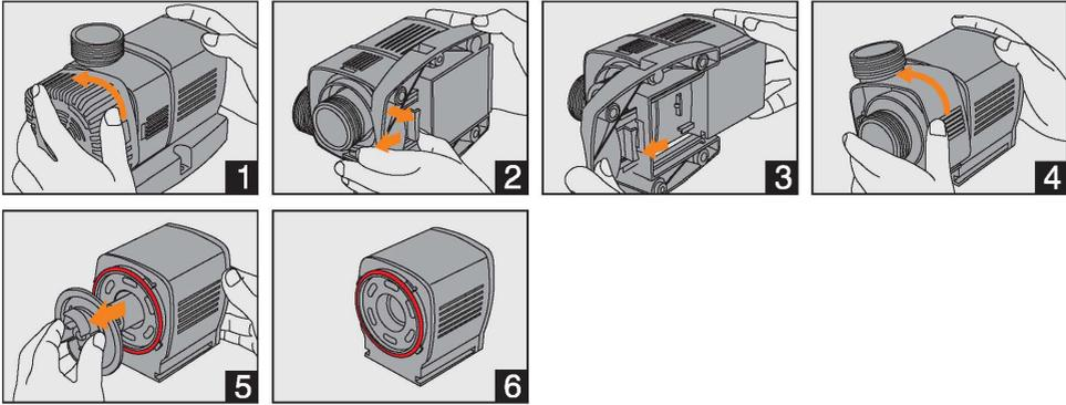
1. Turn the filter case in the direction as indicated by the arrow, then lift it off.
