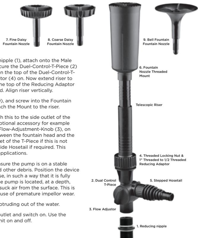
Using the 1" to 1/2" threaded reducing nipple (1), attach onto the Male Threaded outlet of the pump. Now secure the Dual-Control-T-Piece (2) onto threaded reducing nipple. Now on the top of the Dual-Control-T-Piece (2), connect the Reducing Adaptor (4) on. Now extend riser to the desired height, then secure onto the top of the Reducing Adaptor with the threaded locking nut provided. Align riser vertically.
