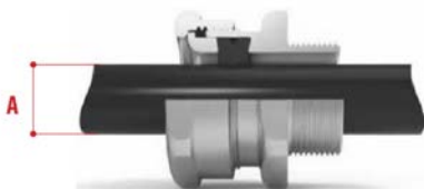
Cable gland with gasket with unarmored cable
