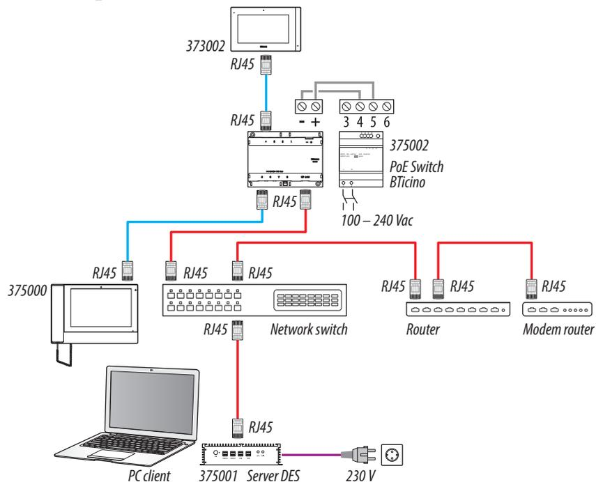
**Attention:** do not directly connect PoE ports to an unsuitable network interface, such as a device powered by a different voltage. Connect the UP LINK port to a suitable port, never to a PoE port.
