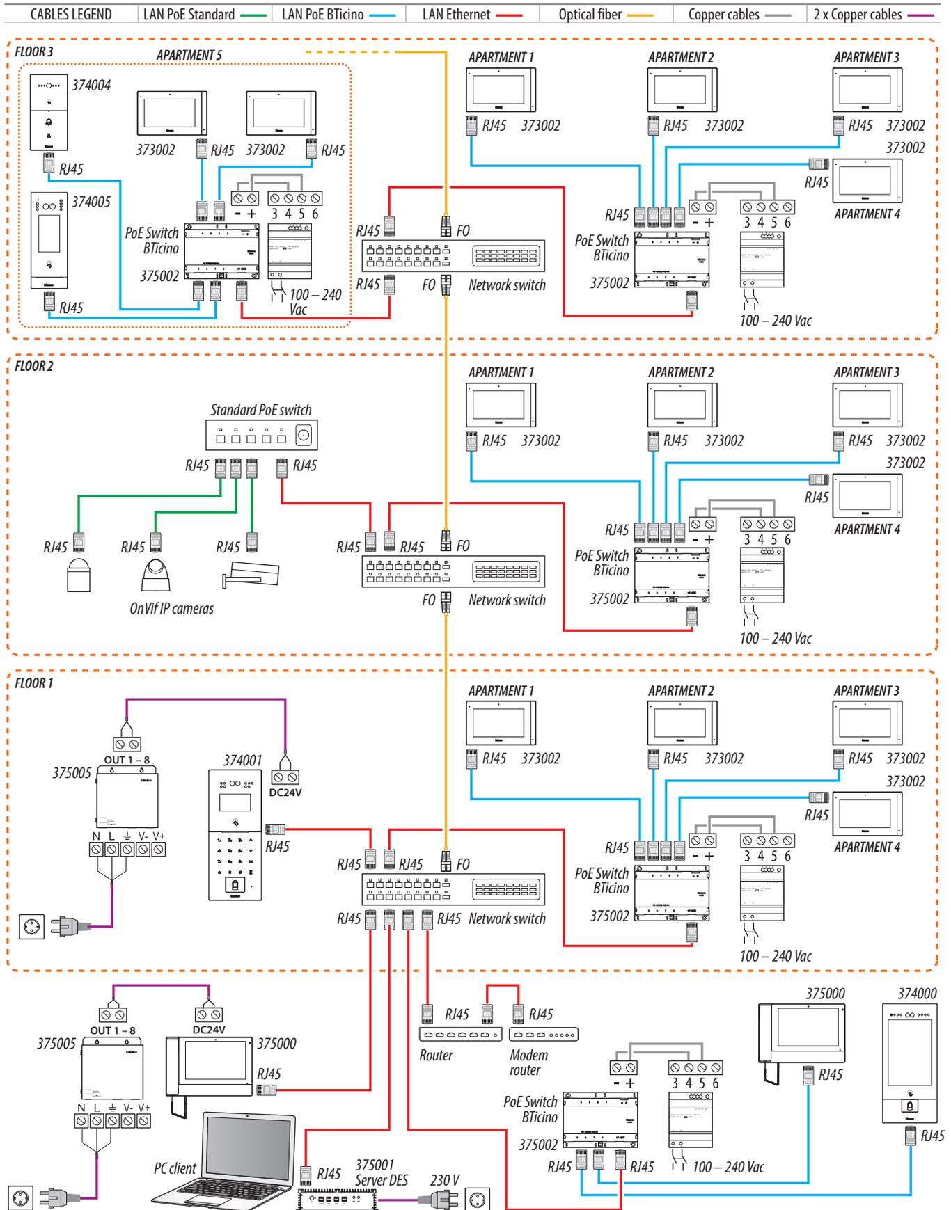
**Attention:** do not directly connect PoE ports to an unsuitable network interface, such as a device powered by a different voltage. Connect the UP LINK port to a suitable port, never to a PoE port.
