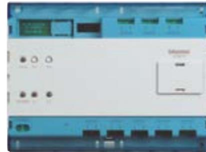
**Lift control interface with 8 relays** to integrate lift function in IP door entry system. The configuration is made directly in IP DES configuration tool included in Server DES.
